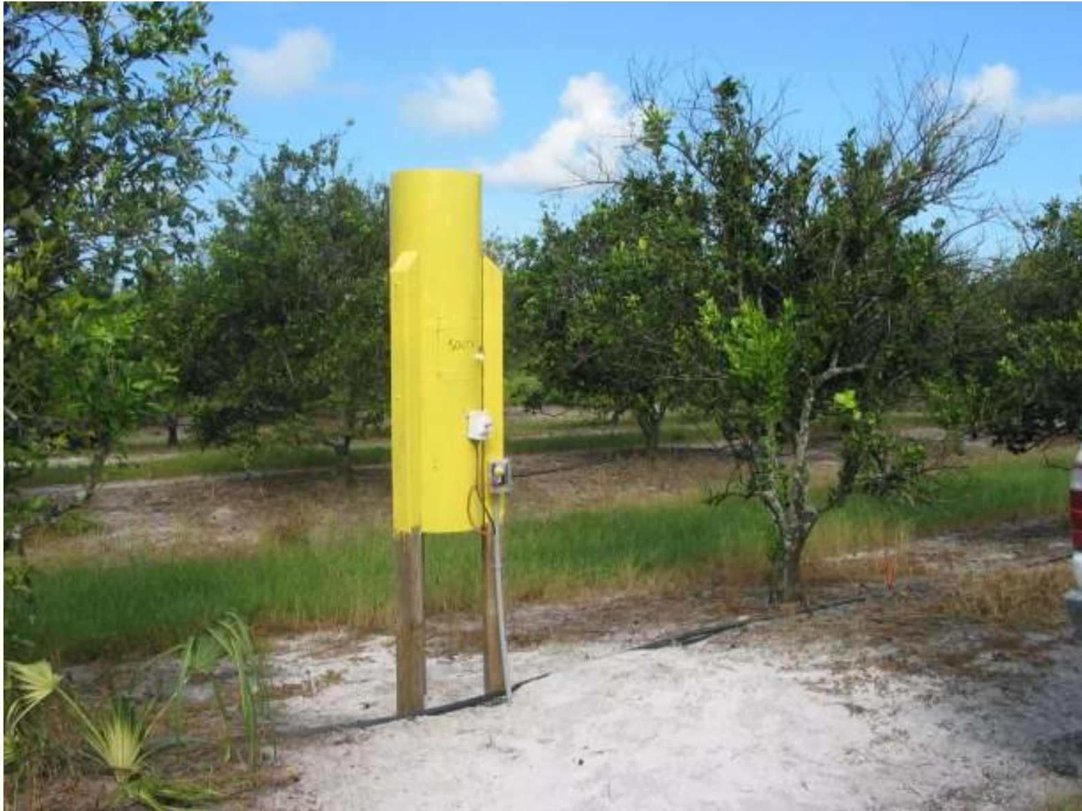
Suction trap for detecting adult psyllids (photo courtesy of Susan Halbert)
